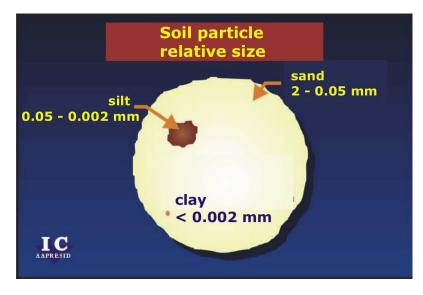
These particles are also together forming aggregates. This property is called **structure**.
